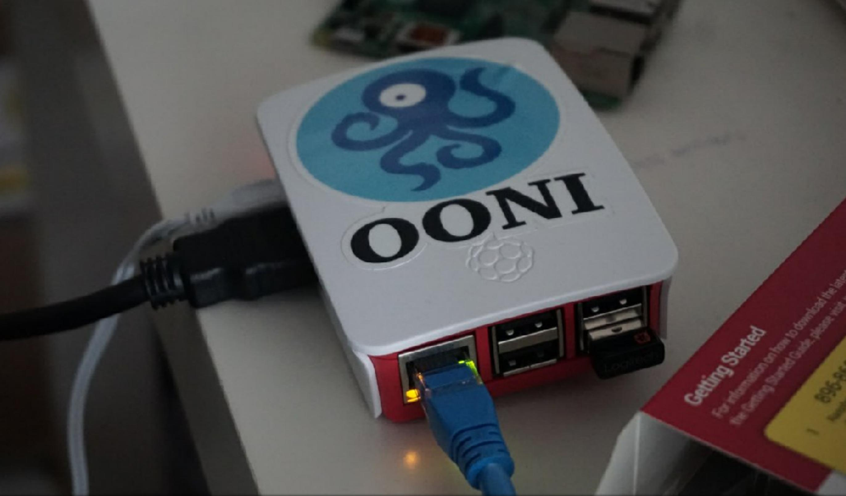
ooniprobe on RaspberryPi
